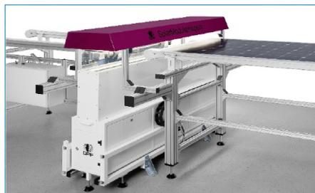
*SolarModuleInspect* detects distances between cells, dimensions of cells, the location of strings as well as connectors. Additionally the system inspects the surface of the PV-module, detecting bubbles inside the EVA foil, inclusions, flecks, marks and many more defects.
