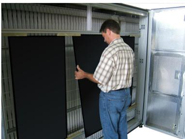
Fig. 1: Atonometrics UV exposure chamber module loading
